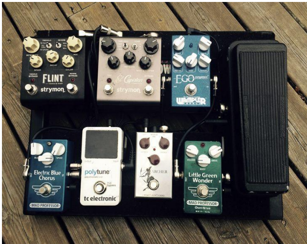
Figure 2: A real pedal board used by guitarists. Pedals are chained together before going to the amplifier.
