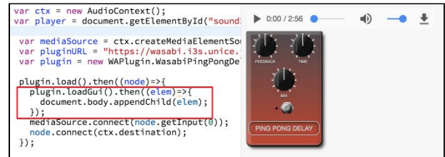
Figure 3: the same plug-in, with GUI. Note that the GUI code is downloaded in the host only when needed 10 .
