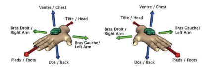
This type of interaction is particularly effective and readable for slow movements. It can also be used for rapid movements, but the perception of speed will be easily translated with the information from the gyro speed sensors. The vector analysis of gyration is not dependent from a particular direction, but the speed of rotation. Accelerometers are also used to detect jolts of movement.
